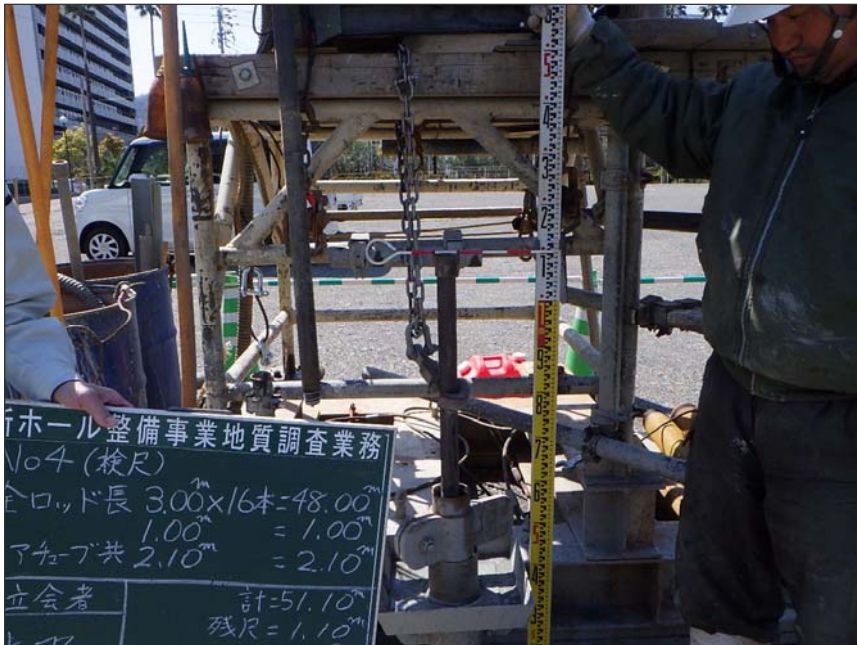
No. 4 削孔長検尺
